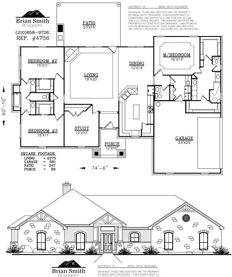
(210)658-9726 REF. #4756 DRAWINGS, PLANS AND SKETCHES ARE THE PROPERTY OF BRIAN SMITH DESIGNERS. PURCHASER'S RIGHT IS CONDITIONAL AND LIMITED TO A ONE TIME USE TO CONSTRUCT A SINGLE PROJECT. PRELIMENARY SKETCHES ARE PROHIBITED AS CONSTRUCTION DAWINGS. UNAUTHORIZED USE OR REPRODUCTION OF THESE PLANS AND SKETCHES ARE STRICTLY PROHIBITED. VIOLATORS WILL BE PROSECUTED.
